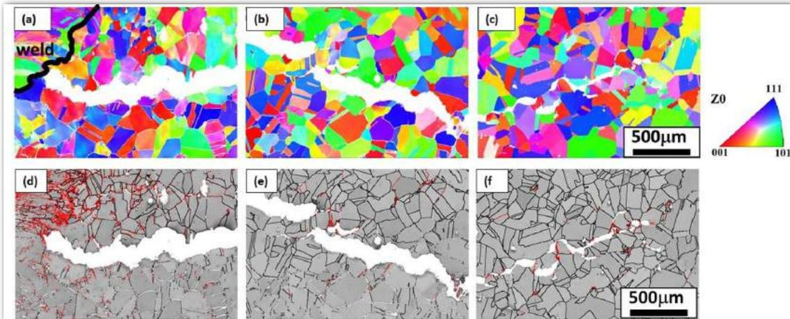
Figure 3 (a-c) Orientation maps and (d-f) grain boundary maps of reheat crack at location 1 (a, d), location 2 (b, e) and location 3 (c, f). Position of each location is marked in Figure 2(a).
