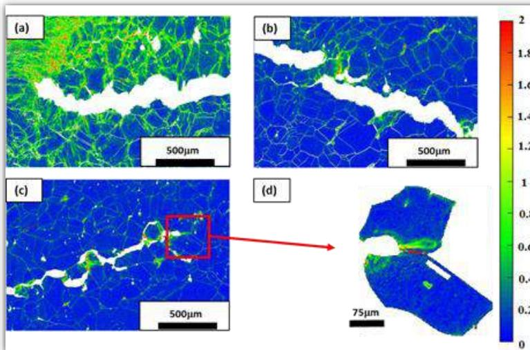
Figure 4 - Kernel average misorientation (KAM) maps of the reheat crack at (a) location 1, (b) location 2, (c) location 3 and (d) magnified map of grains at the crack tip.
