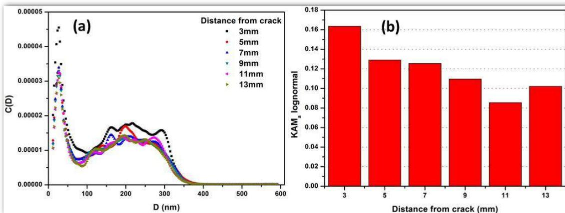
Figure 5(a) SANS data showing the increase in fractional size distribution of cavities and (b) EBSD data showing higher values of  $KAM_a$  lognormal, as approaching the crack, along a line normal to the crack.
