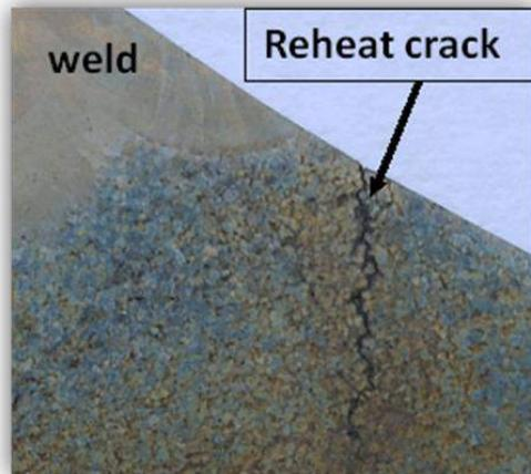
Figure 1: Reheat crack near a weld in 316H stainless steel.
