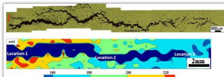
Figure 2 (a) Optical microstructure and (b) hardness map around the reheat crack.
