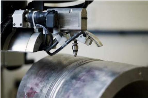
Figure 1: X-ray diffraction probe measuring a welded pipe.
